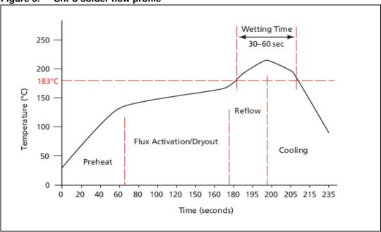
Figure 7. Pb-free solder flow profile
