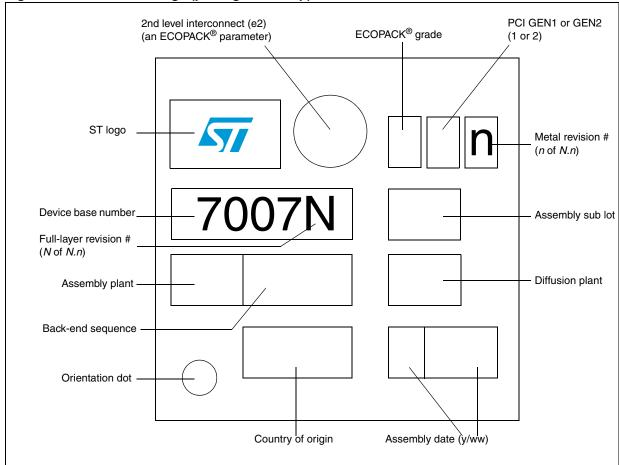
In order to meet environmental requirements, ST offers these devices in different grades of ECOPACK<sup>®</sup> packages, depending on their level of environmental compliance. ECOPACK<sup>®</sup> specifications, grade definitions and product status are available at: <a href="https://www.st.com">www.st.com</a>. ECOPACK<sup>®</sup> is an ST trademark.
